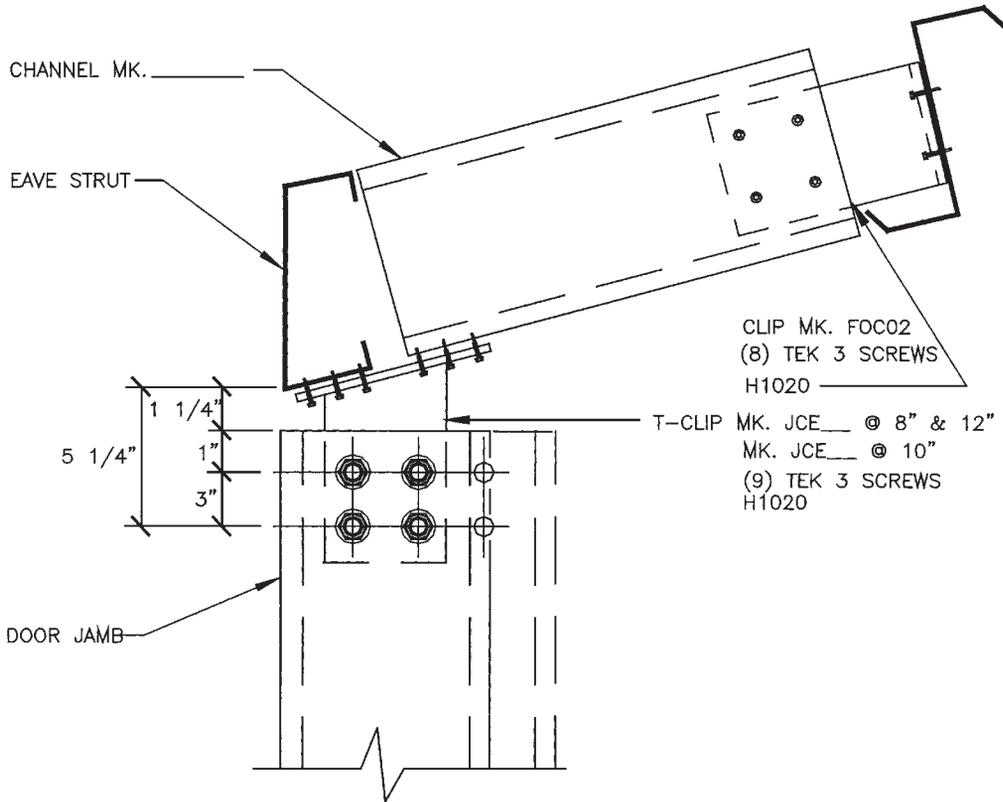
**FIGURE 10.8** Connection of door jamb to braced eave strut. [Manufacturer suggests using (4) 1/2-in ASTM A307 bolts.] (Nucor Building Systems.)
